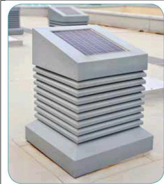
Figure 5.30. Modern windcatcher Sola-Boost by Monodraught, UK. It is divided into four sections, working bidirectional at all wind directions. Integrated there's a 10W monocrystalline photovoltaic solar module, linked to an assisting fan (2W at nominal power), adding up to 35l/s in addition to 110l/s ventilation calculated at between 2 and 3 m/s external wind speed. Source: http://www.monodraught.com (20.04.2014)
